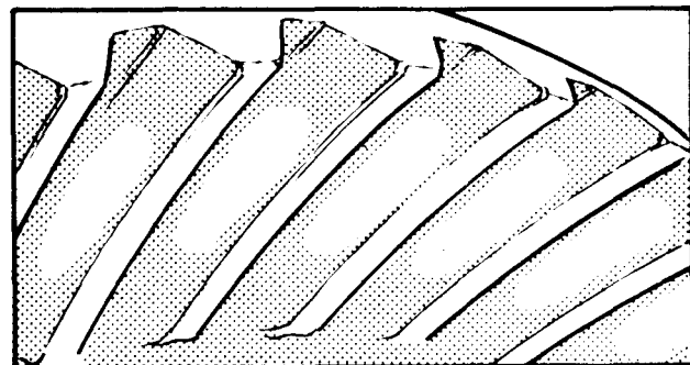
PATTERN "C" - CONCENTRATED BEARING AT HEEL
